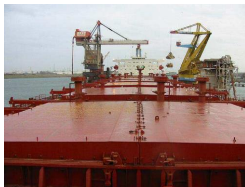
A hatch or hatchway is the opening at the top of a cargo hold.
